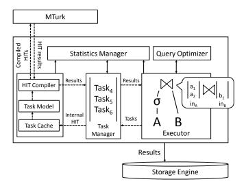
Figure 1: A Qurk system diagram.
